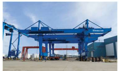
Rail Mounted Container Gantry Crane
